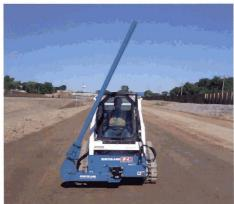
The EZR quickly and easily mounts on any skidsteer. And its Hydraulic Actuator allows the Stem to swing 180 degrees left or right, as well as angle 115° up and 8° down. Stem is detachable and available in three lengths.
