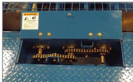
Easy maintenance access to roller chain drive and bearings. Heavy duty, greasable, cast steel flange bearings.
