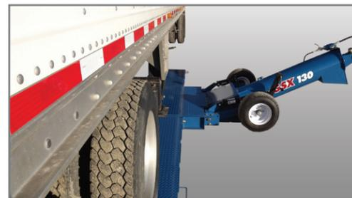
The GSX's extended, tread plate platform leaves room to safely step across the hopper while the truck is parked over it. This leaves extra room to turn the trap door crank and extra room for a trailer that may not be perfectly straight behind the truck. Transport wheels and optional hydraulic lift are placed low and out of the way. This feature saves time and steps every time a truck is dumped.
