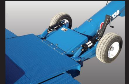
Hydraulic lift. A jack is used on standard machines.
