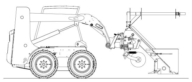
Units equipped with a sliding offset hitch and skid steer adapter are also stored with the hitch on the ground. Always lower the silt fence installer to the ground when not in use. Never enter or exit the loader cab with the boom in the raised position.
