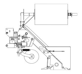
Load the fabric onto the roll mount tube.
