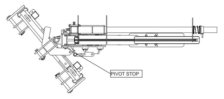
The silt fence installer pivots 40 degrees from centerline between the hitch and the frame. This allows the machine to install tight radius curves in the silt fence installation. There is a pivot stop on the hitch of the silt fence installer. Do not continue to turn the tractor or skid steer after the silt fence installer has reached the pivot stop. Oversteering the machine may cause the silt fence installer blade to bend. Blades bent from oversteering are not covered by warranty.
