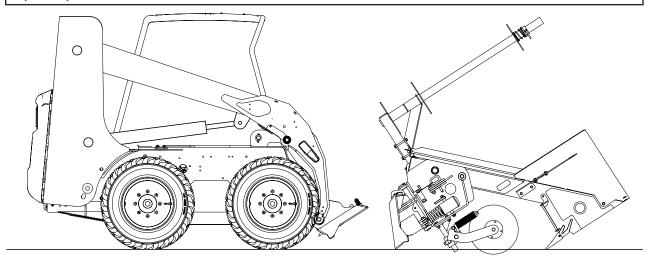
Raise the loader boom and make sure the silt fence installer is securely resting on the loader attachment plate. Follow the instructions in your loader operator manual to extend the attachment locking pins and lock the attachment in place.
