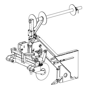
Store the stands above the sliding offset hitch on installers equipped with a sliding hitch.
