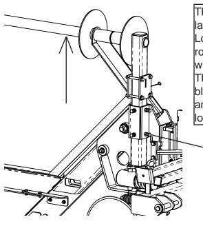
The roll holder can be raised to accomodate large diameter 42 in. or 48 in. rolls of material. Loosen the jam nuts and lock bolts to raise the roll holder. Tighten the lock bolts and jam nuts when the roll holder is at the desired position. The roll holder height should be kept low if possible. Material is easier to load on a low roll holder and the center of gravity of the machine will be lower.
