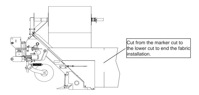
The fabric can also be cut completely above the chute. The method shown above does not require the fabric to be re-threaded after the cut.
