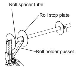
The silt fence installer can install 36 in., 42 in., and 48 in. wide fabric. The machine is configured to install 36 in. fabric as shown. To install 42" fabric, remove the roll holder gusset and replace the roll stop plate. To install 48" fabric, remove the roll stop plate, roll holder gusset and roll spacer tube. See the parts section for a detailed breakdown of the roll holder assembly.
