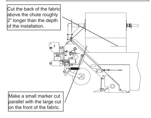
After the cuts have been made, pull the installer forward until the cuts are behind the fabric chute.
